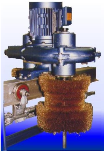
OP-8 conveyor chains and equipment for cleaning of bearing drums
